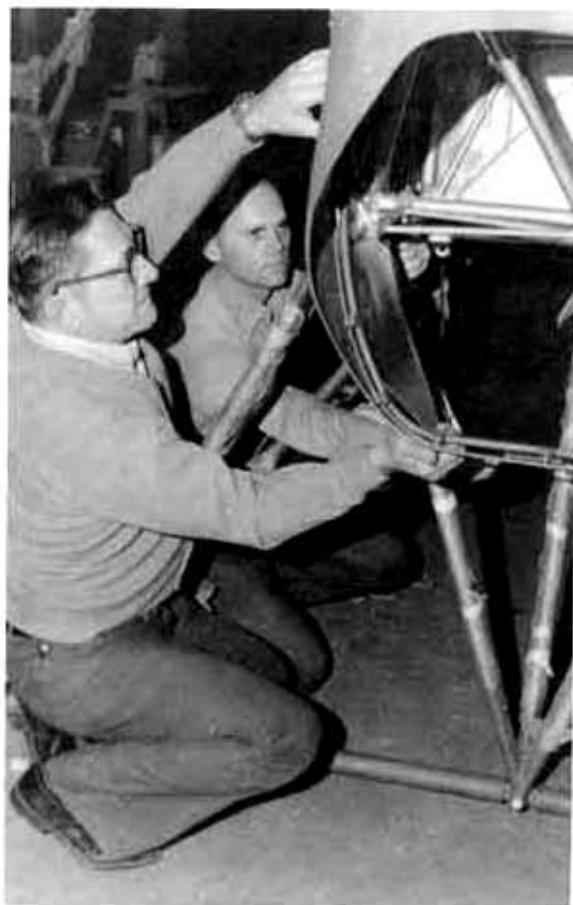
Mr. Alex J. Sekulich (l) and GySgt Gary L. Johnson check a handmade FB-5 cowling panel for fit. The evolution of a flat paper engineering drawing into its final compound-curved aluminum form requires many such checks.
